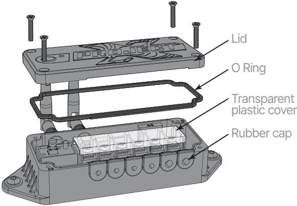
Cut the pointed head of the Rubber Caps according to the thickness of the hardwire cable.
