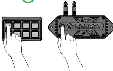
7. Press the pair button on the Ghost Box and any one of the 8 device buttons on the Keypad together and hold for 3 seconds. If the App screen shows a new device is added, that means the pairing of the Ghost Box, Keypad and the App is successful. You can start customizing your 12V accessories.
