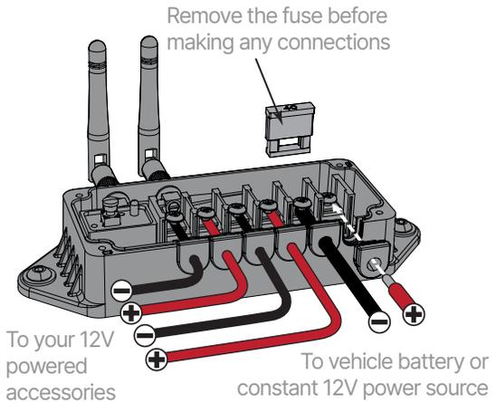
\*Suggested gauge of wire for direct connection: 10 AWG
